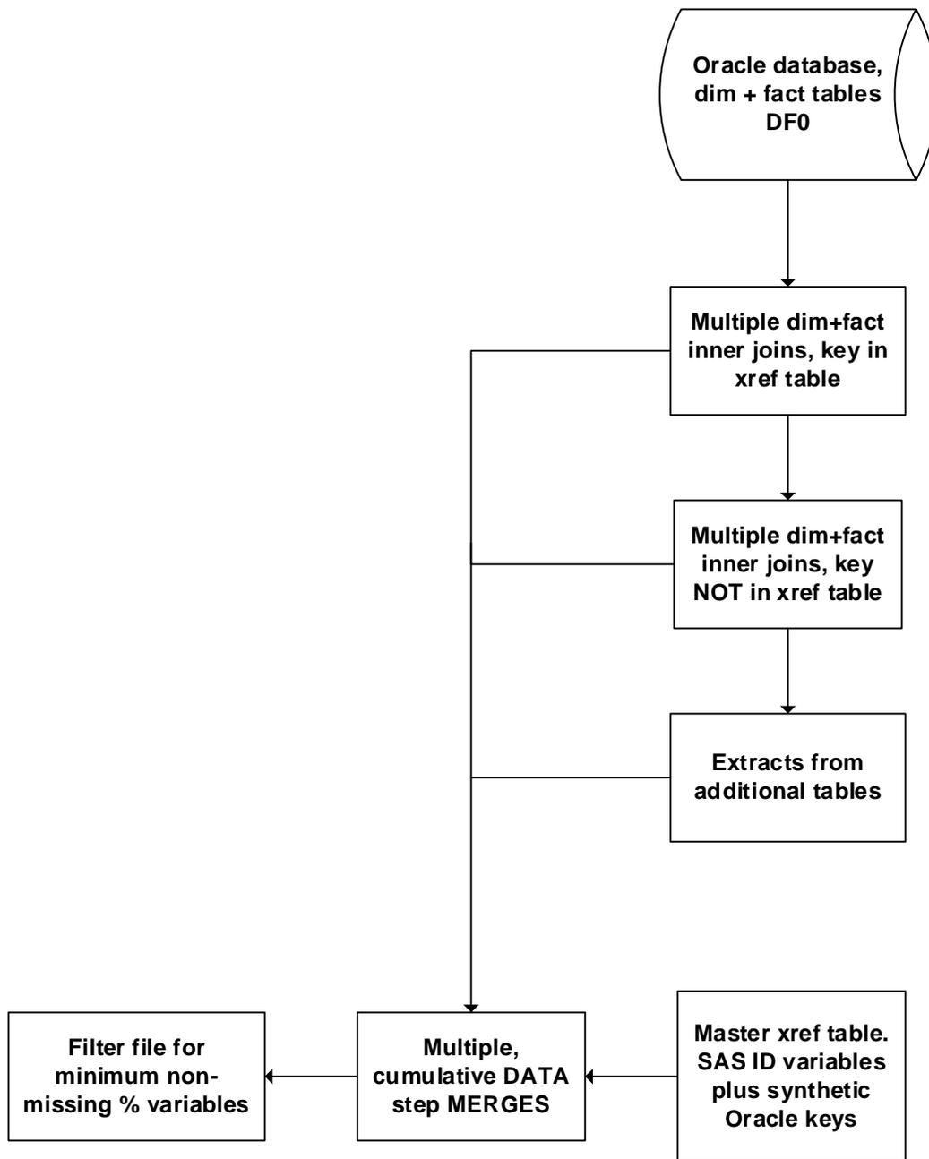
Figure 2. Monthly processing for omnibus file
